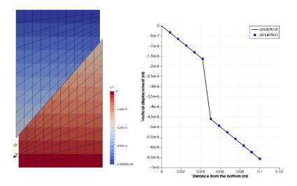
Figure 1.2: Deformation result (left) and profiles of vertical displacement at  $x=0.2~{\rm m}~({\rm right})$
