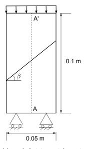
Figure 1.1: Problem definition with an inclined fracture
