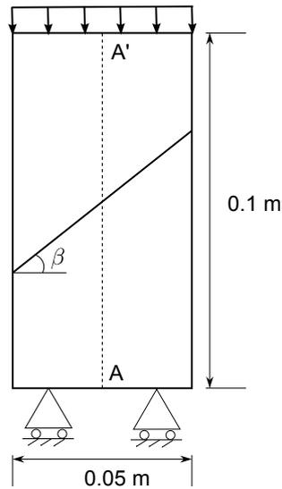
Figure 1.1: Problem definition with an inclined fracture
