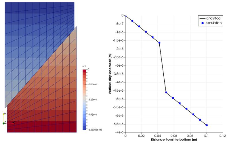
Figure 1.2: Deformation result (left) and profiles of vertical displacement at  $x = 0.2$  m (right)
