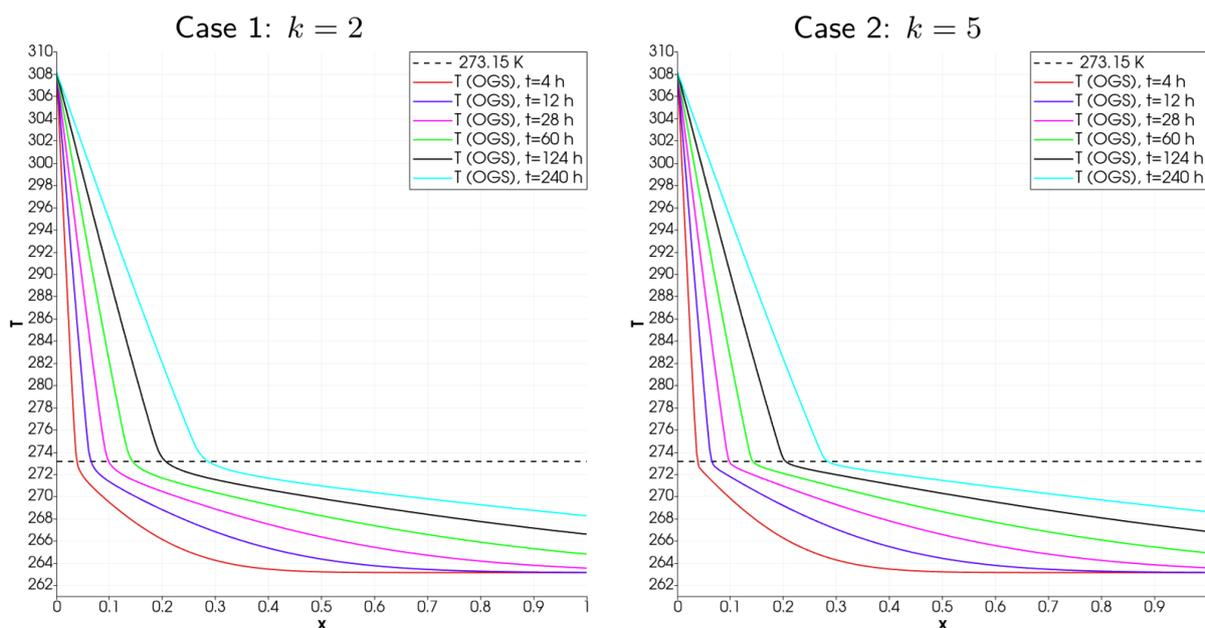
Figure 4: The OGS solution of the IBVP for the T+freezing equation (1) at time-steps  $t \in \{4 \text{ h}, 12 \text{ h}, 28 \text{ h}, 60 \text{ h}, 124 \text{ h}, 240 \text{ h}\}$  in the interval  $x \in [0, 1 \text{ m}]$  for the two cases of  $k$ ; temperature is given in kelvins.
