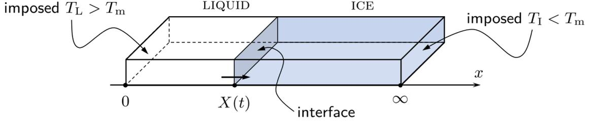
Figure 2: Sketch of a semi-infinite melting slab as a physical situation modelled by the two-phase Stefan problem.
