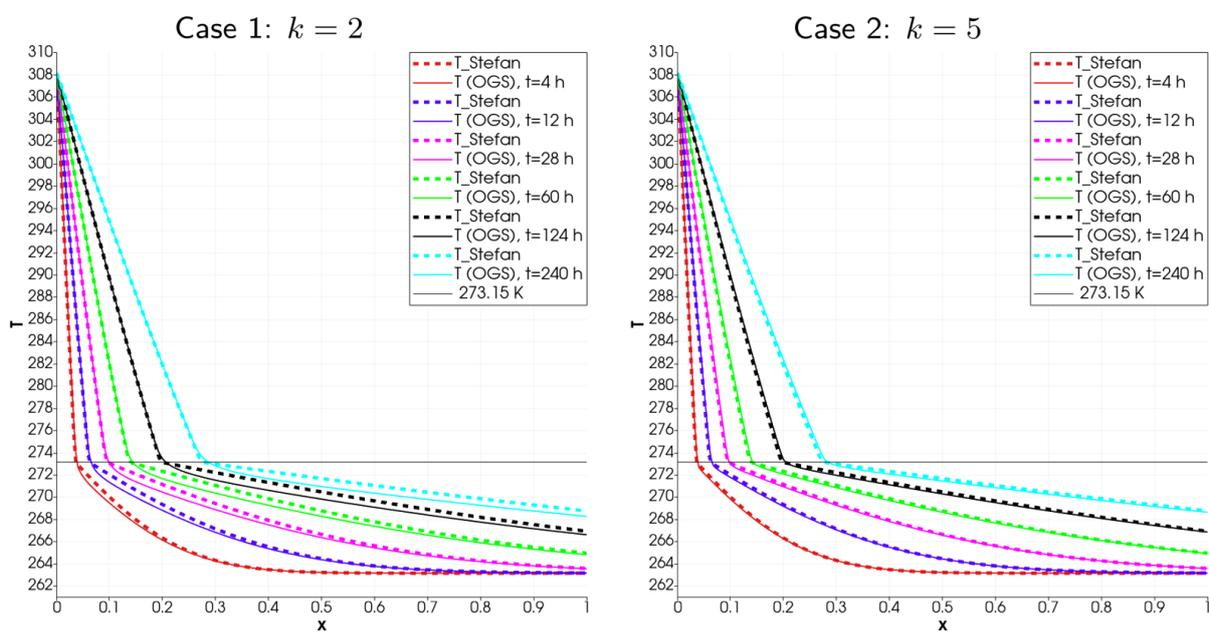
Figure 5: Comparison of the analytical solution (4) to the two-phase Stefan problem and the OGS solution to IBVP for for the T+freezing equation (1) obtained in two cases of  $k$ ; the temperature is given in kelvins.
