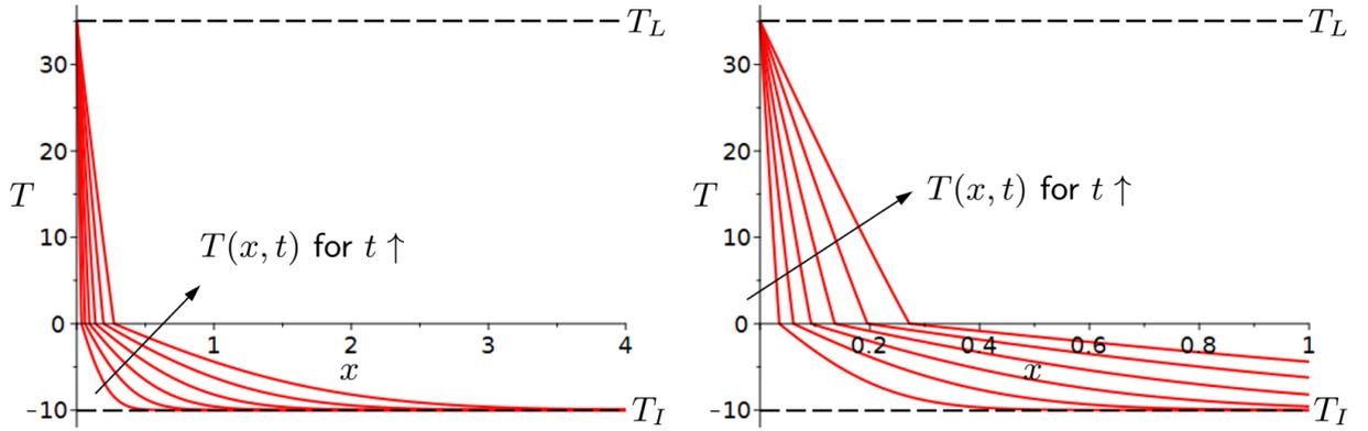
Figure 3: Solution (4) at time-steps  $t \in \{4 \text{ h}, 12 \text{ h}, 28 \text{ h}, 60 \text{ h}, 124 \text{ h}, 240 \text{ h}\}$  in the intervals  $x \in [0, 4 \text{ m}]$  (on the left) and  $x \in [0, 1 \text{ m}]$  (on the right); dashed lines depict the prescribed  $T_L$  and  $T_I$  in degrees Celsius.
